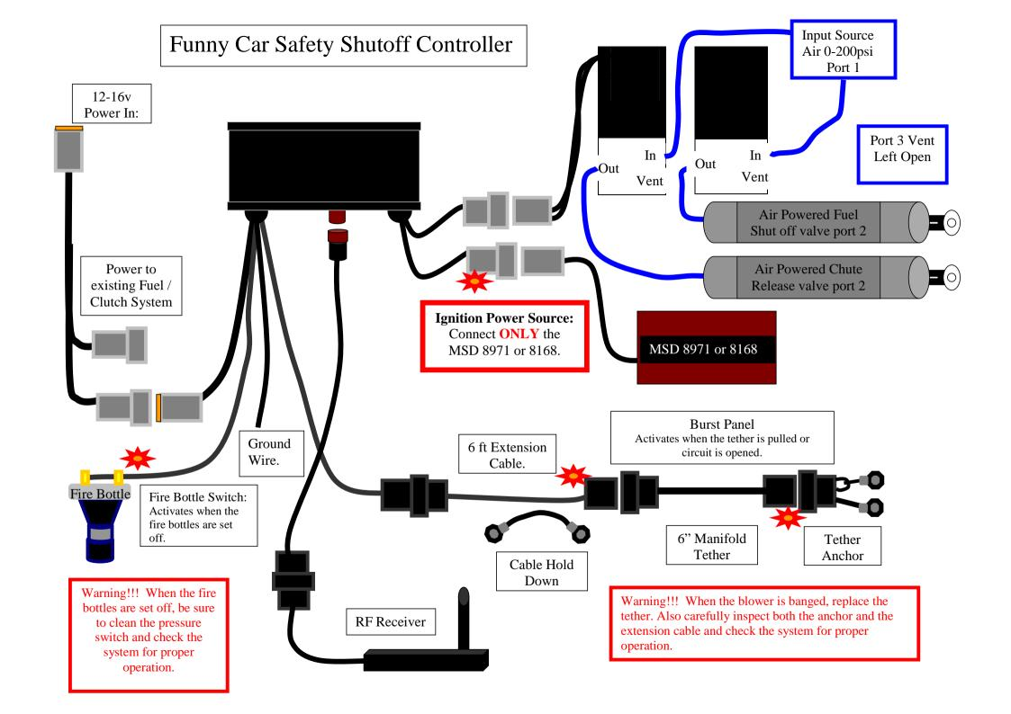
The Electrimotion Safety Shutoff box is designed to shut off the car as a result of a catastrophic event. The box has 3 trigger inputs, which will trigger 3 separate output events. The 3 trigger inputs are a burst panel input; a Fire Bottle trigger input and a wireless shut down input.
