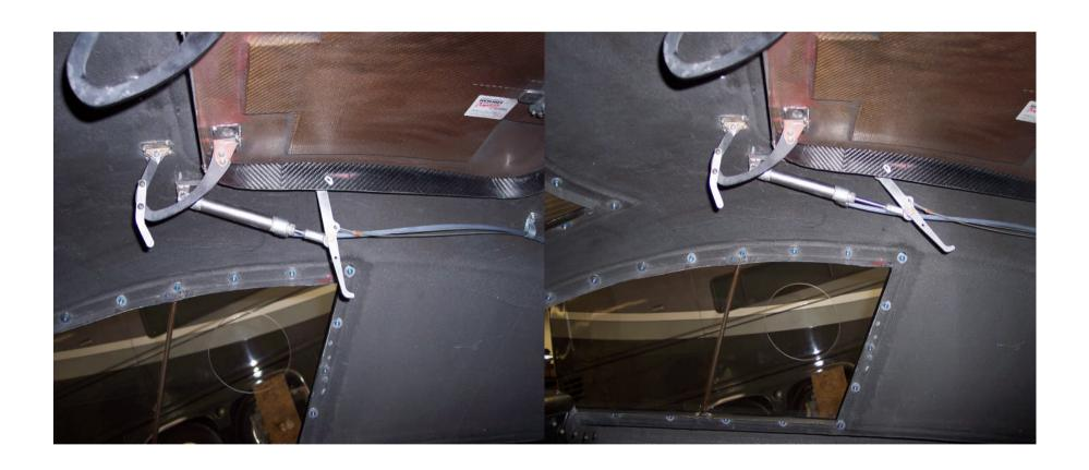
Typical Mounting of Fire Bottle Air Switch.
