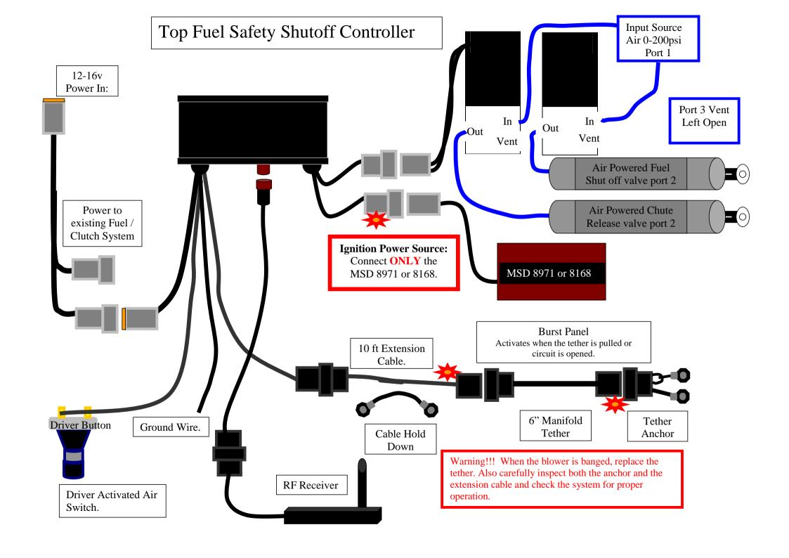
The Electrimotion Safety Shutoff box is designed to shut the car off as a result of a catastrophic event. The box has 3 trigger inputs, which will trigger 3 separate output events. The 3 trigger inputs are a burst panel input, an air activated driver push button trigger input and a wireless shut down input.
